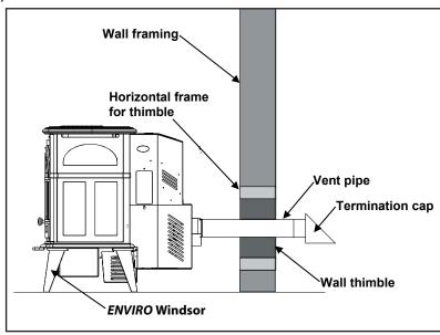
Figure 10: Straight through Wall Installation - Side View.
